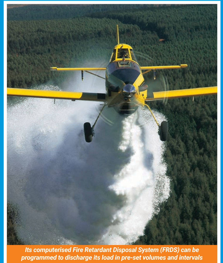
The AT 802 carries up to 3 104 litres of water, mixed with fire suppressants, reaching a cruising speed of 250km/h for rapid response to a fire line
